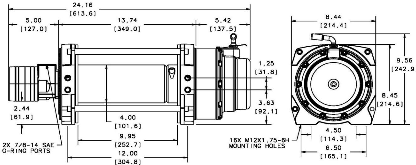
Motor / Contactor may be rotated in 90 degree increments. Clutch housing may be rotated in 72 degree increments.
